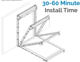
The RollSeal WIC door comes with 3 main components: the head unit and two tracks. The three components are assembled in front of the door opening using three bolts on each side of the door. Once the door is lifted into place it can be fastened to the wall. All electrical components are pre-wired with CPC connectors. Electrician required to bring power to one location and then start up can begin.
