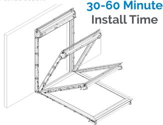
The RollSeal WIF door comes with 3 main components: the head unit and two tracks. The three components are assembled in front of the door opening using three bolts on each side of the door. Once the door is lifted into place it can be fastened to the wall. All electrical components are pre-wired with CPC connectors. Electrician required to bring power to one location and then start up can begin.
