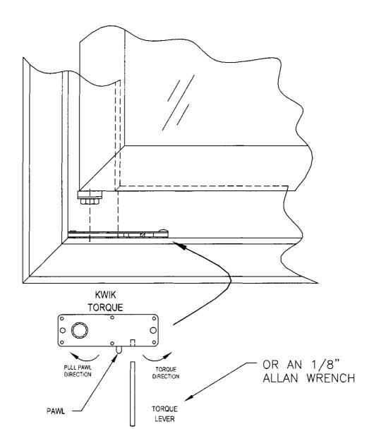
WITH DOOR IN CLOSED POSITION, YOU WILL ENGAGE THE TORQUE OPERATED SELF CLOSING MECHANISM:
