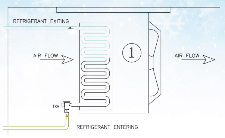
The Latent heat required to boil off this refrigerant from a liquid to a gas is taken from the air as it passes through the coil, thus cooling the air. This boiling process is called evaporation, thus the coil in which this occurs is referred to as our evaporator. The evaporator is where we collect the heat we want to remove.
