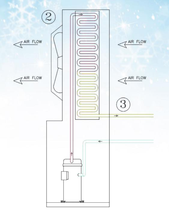
The latent heat required to condense this gas is rejected from the refrigerant into the outside air. This process is called condensation, thus the coil which this occurs is referred to as the condenser. The temperature that the condensation occurs is much higher than within the evaporator, as the pressures in the condenser are much higher.
