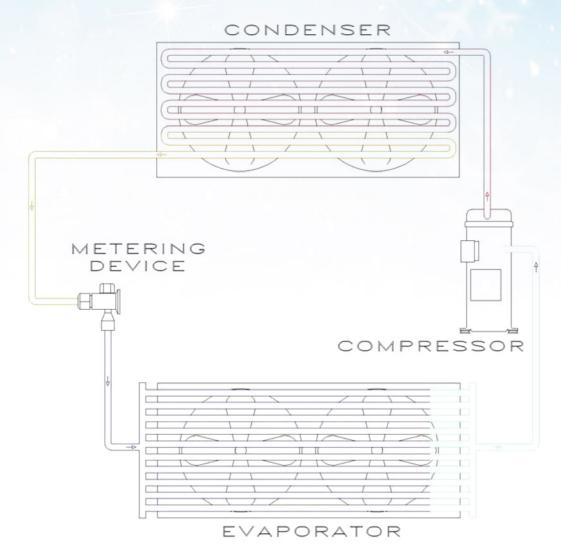
**What is Refrigeration?** Refrigeration is simply cooling by removing heat. Heat is a form of energy that can't be destroyed. Therefore to remove heat we can only transfer from one place to another. Even though it is easier to think of refrigeration as the process of making things cold, it actually is the process of transferring heat from one place to another.
