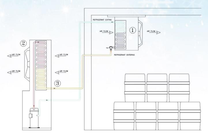
In review, we removed the heat from the room by transferring the heat from the air into the refrigerant (1). The refrigerant carried this heat to the outdoor air cooled condenser, then this heat was transferred from the refrigerant to the outside air (2).
